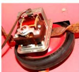
It runs by a small motor under the base which turns a wheel which turns the big wheel.
